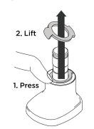
2.3 Replace rotation ring in the desired orientation.
