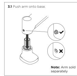
**3.2** Ensure arm is fully pushed onto base.
