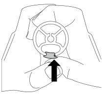
**B.** Press down firmly onto the other edge of the Cable Stop and hold. This allows the rear profile to flex in place.
