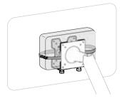
This product adds an additional 2 lbs. (1 kg) to your mounting solution. When mounting between a monitor and VESA plate, the mounting solution's monitor weight capacity must be reduced by 2 lbs. (1 kg) when using standard monitors and thin clients which when combined are less than or equal to 2.5" (64 mm) thick. Additional reduction will be required if the combined monitors and thin client are greater than 2.5" (64 mm) thick.
