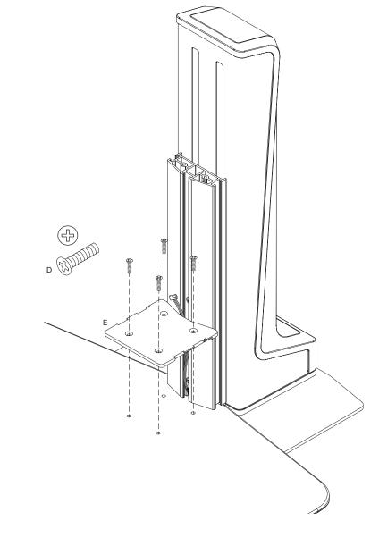
3 4 Place the utility tray on top of the work surface by aligning the (4) tabs on Proveno utility tray with recessed areas on work surface plate. With the tabs aligned, slide utility tray towards the column to secure into place.
