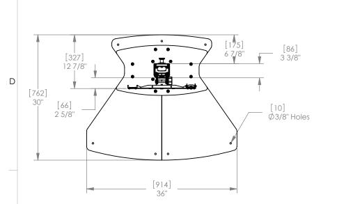
NOTE: CUSTOM INTERAFCE BRACKET NOT SHOWN. THE CUSTOM INTERFACE BRACKET NEEDED FOR YOUR DISPLAY WILL ADD BETWEEN 1/2" AND 2" IN DEPTH AND MAY AFFECT LOCATION OF DISPLAY ON THE MOUNT.
