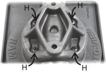
11. DETERMINE PROPER HEIGHT ADJUSTMENT BY SLIDING (N) TUBE UP AND DOWN AS NEEDED. WHEN SET TO THE CORRECT POSITION, EVENLY TIGHTEN THE (H) SCREWS BEHIND (A) ROTO-VIEW™
