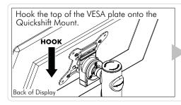
Press and hold the Release Buttons. Gently push bottom of VESA Plate into Quickshift Mount. Release Buttons to lock in place.
