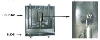
5.) EXPAND (D) SPRING UNTIL SCREW FROM STEP 4 ALIGNS WITH HOLE IN TRAY HOUSING. TIGHTEN SCREW THROUGH HOLE WITH (J) NUT POSITIONED ON OPPOSITE SIDE.
