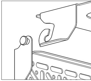
**3.2** With latches in open position rotate Tray **B** until parallel with mounting surface.
