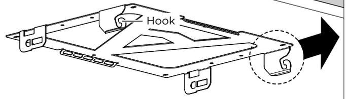
**Exposed configuration bracket orientation**
