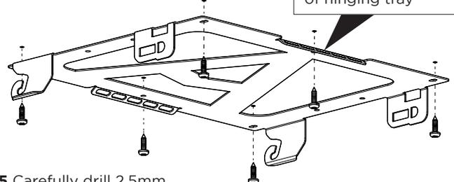
**2.5** Carefully drill 2.5mm (3/32") pilot holes. Fasten Bracket with Wood Screws **C**. Do not overtighten.
