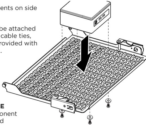
**Tip:** Use Washers **E** when using component fasteners if needed
