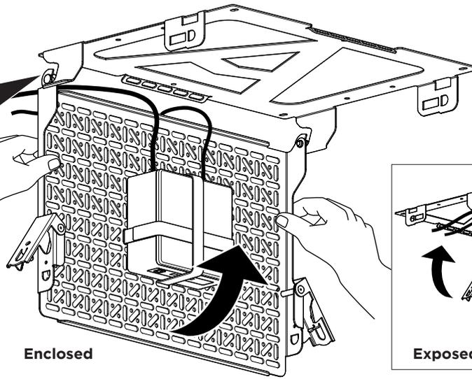
**NOTE:** Cables must always exit at the hinging side of tray
