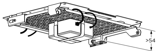
**2.1A** Position hooks towards back to make components accessible when tray hanging for maintenance.
