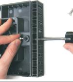
3. WITH SPRING WEDGED IN PLACE, ATTACH (N) SCREW THROUGH COUNTERSUNK HOLE. ONCE TIGHTENED, REMOVE (K) SCREW FROM SPRING.
