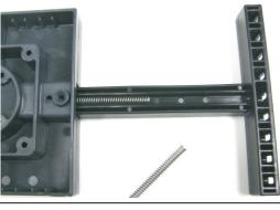
2. COMPRESS SPRING INTO TRAY USING A PHILIPS HEAD SCREW DRIVER. WHEN SPRING REACHES PAST COUNTERSUNK HOLE, WEDGE SPRING IN PLACE WITH (K) SCREW.
