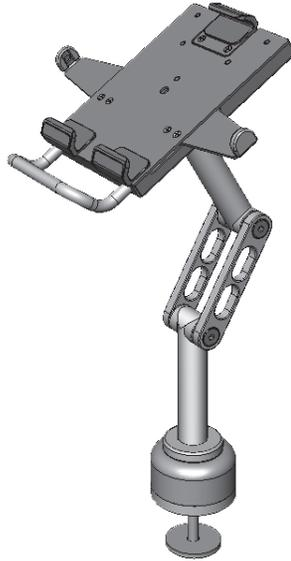
Screw 3/8 All Thread bolt into offset hole in base of desk mount. The bolt is included in the hardware bag.
