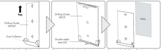
Un-fold the Drilling Guide and Peel away the backing from the open the Dust Collector.
